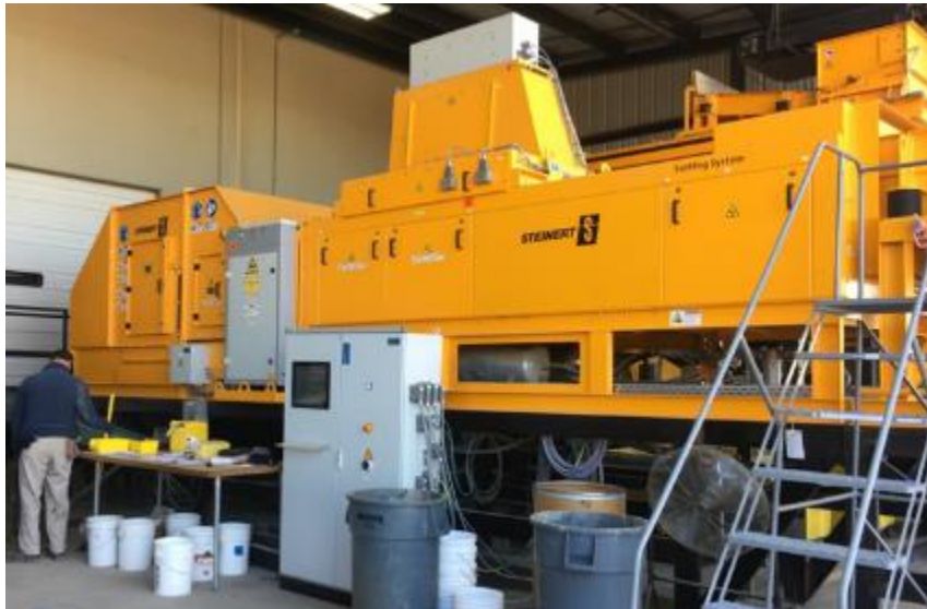
Figure 13-16: Steinert KSS CLIXT Sorter
