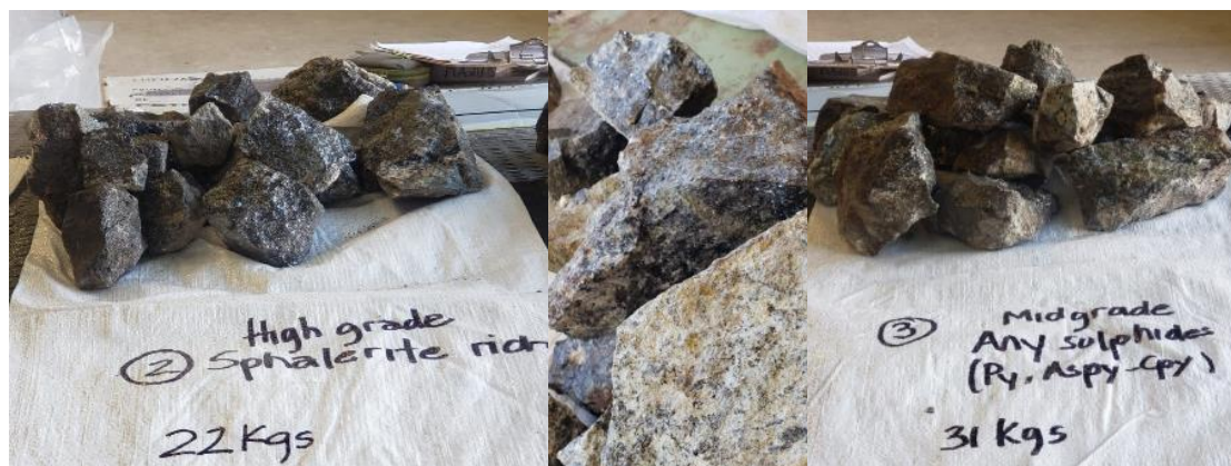
Figure 13-6: Sphalerite Rich (2) – Mid Grade (3), Other Sulphides: Chalcopyrite, Pyrite and Arsenopyrite
