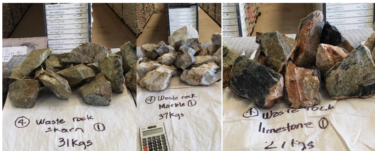
Figure 13-7: Skarn, Waste Rock Marble, Waste Rock Limestone, Waste Rock
