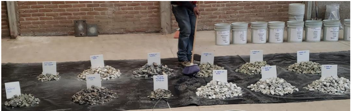
Figure 13-11: Crushed Specimens Prior to Blending
